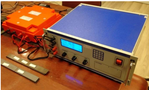
The Epstein tester with the Epstein bridge.
